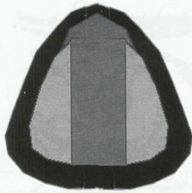
Fig.7. Typical limb cross-section showing addition of the horn plate at the belly (top), forming a sharp apex along the belly.
